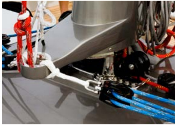
Rotating carbon mast provides optimum aerofoil shape for fully battened mainsail.
