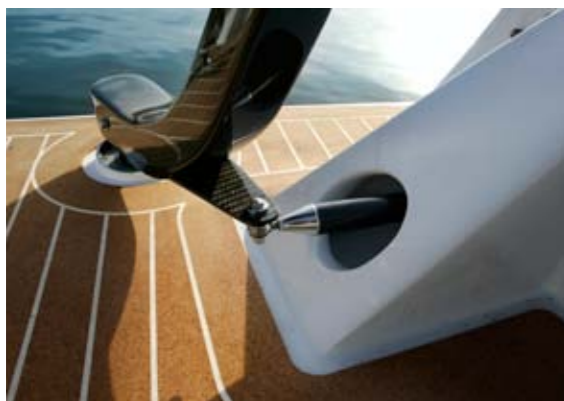
Finger light steering thanks to self-aligning bearings and direct linkage.
