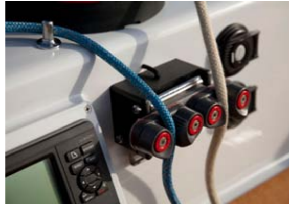
Sails can be automatically released by an anti-capsize device, should pitch or heel thresholds be exceeded.
