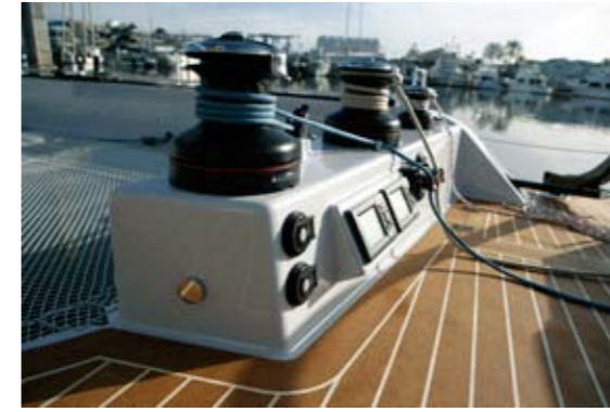
Sheet winches and navigation instruments (including autopilot) are within easy reach of the helmsman).
