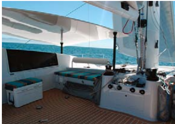
All furling, reefing and mast rotation lines and halyards are led to the mast base. No lines run across the decks, making for a safe environment for non-sailing guests.
